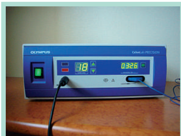
FIGURE 2 : RFITT® unit. Visible settings: power (watts) and duration of application (minutes and seconds in total).
