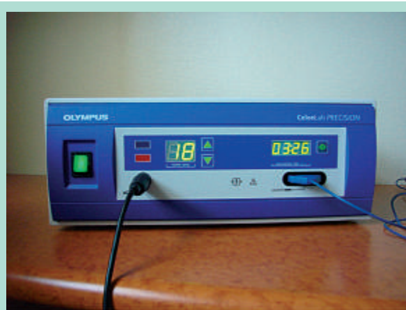
FIGURE 2 : RFITT® unit. Visible settings: power (watts) and duration of application (minutes and seconds in total).
